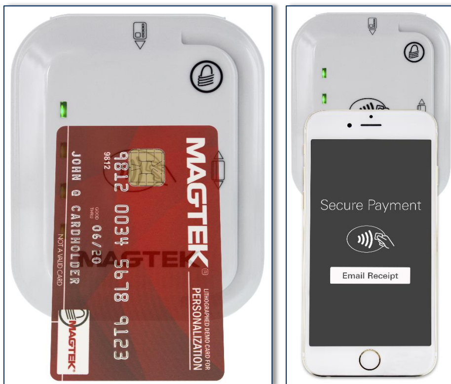
Figure 3-4 - Tapping a Contactless Card or Smartphone On tDynamo
