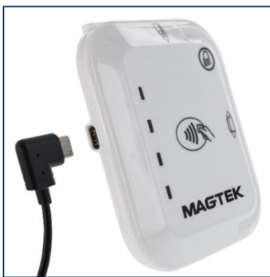
Figure 2-1 - Connecting tDynamo to a Host via USB
