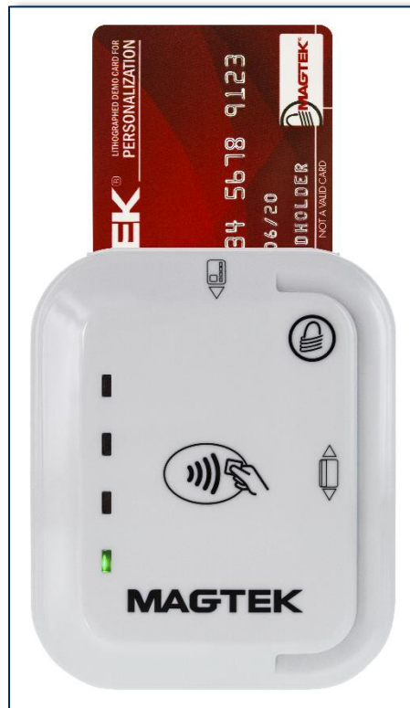
Figure 3-3 - Inserting a Chip Card Into tDynamo
